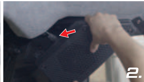
2. Pull off the speaker and unplug from the OEM plug
