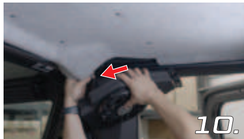
10. Place enclosure back into the vehicle and plug in before securing to the roof
