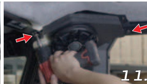
11. Use the same OEM screws to secure the enclosure to the roof
