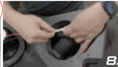
8. Plug in the speaker to the OEM plug
