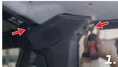
1. Remove the two screws shown here
