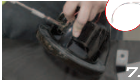
7. Connect the speaker wire harness to the UTV Stereo Speaker
