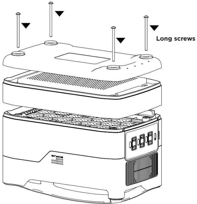
**3.** Align the male and female battery sockets and connect them. Close the bottom cover. Take the four long screws from the Extra Battery Module Kit and screw them securely into place.
