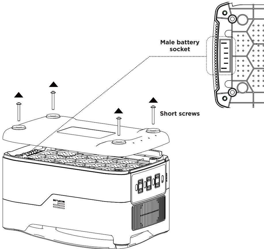
**2.** Unscrew the four short screws according to the figure above before removing the bottom cover. The Male Battery Socket will be visible. Position the Extra Battery according to the figure below. (Note: Do not remove the top cover; only the bottom covers needs removing).
