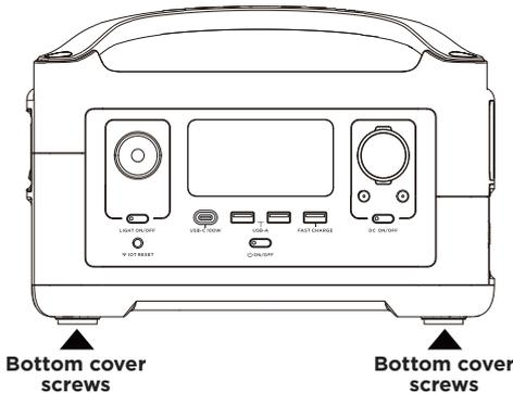
1. Make sure that the RIVER Plus is turned off. Take out the screws from the Extra Battery Module Kit and locate the four screws on the bottom cover.
