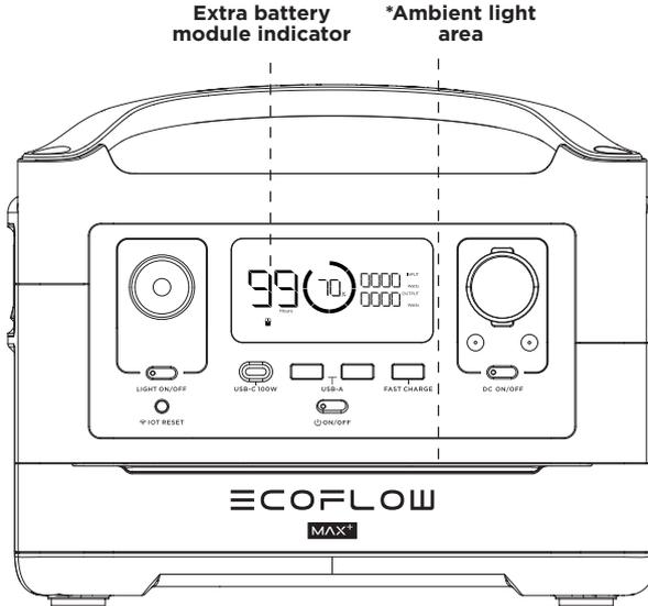
**4.** Turn the RIVER Plus upright and turn it on. The Extra Battery Panel will turn blue. The Extra Battery Indicator will be shown on the RIVER Plus display when it has been installed correctly. Make sure the product is fully charged before use. If the ambient light does not turn on, or the Extra Battery Indicator does not show on the RIVER Plus display, repeat Step 2 and check the product connection.
