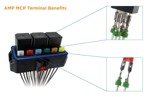
6.3 mm AMP MCP terminal establishes multiple points of contact on both sides of each ISO relay blade terminal, providing stable electrical connection and solid relay retention performance; while 3-gland wire seal provides redundant and robust sealing characteristics to wire and plastic housing.
