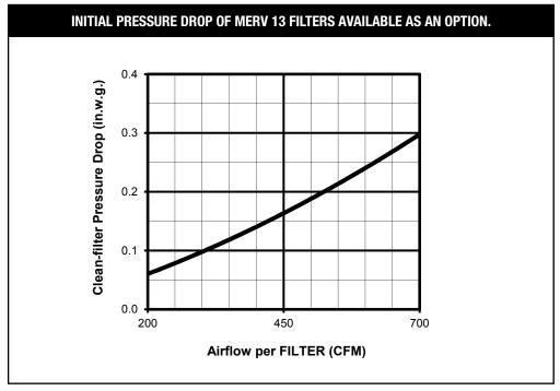
NOTE: pressure drop of standard filter supplied is included in unit airflow performance tables
