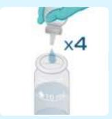
Prepare the sample by adding 4 drops of the Fluoride Liquid Reagent and stir to mix.
