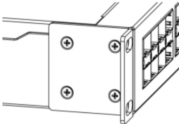
2. Place the device in rackmount enclosure and align with the holes so that the device fits conveniently.
