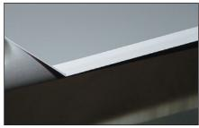
D. Standard Hem. Hems can be formed on all Mark Series<sup>™</sup> brakes, TrimMaster<sup>®</sup> brakes and Metal Master<sup>®</sup> 20 brakes. Visit www. van-mark.com for more tips and ideas.
