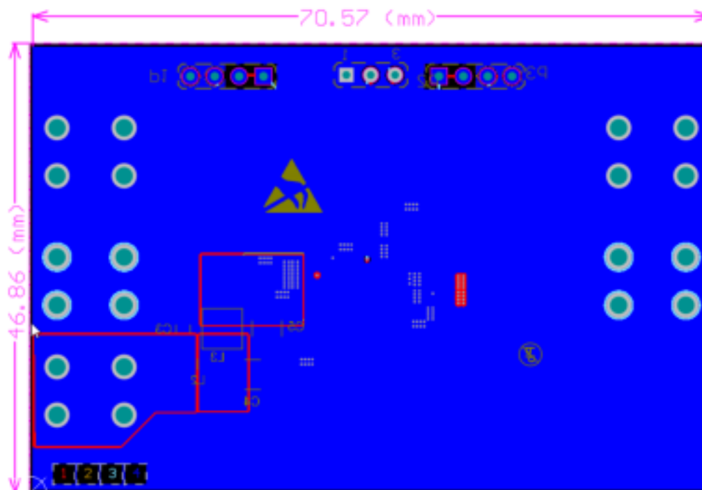
Figure 7. STEVAL-3601CV1 bottom layer
