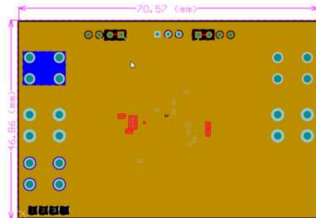
Figure 5. STEVAL-3601CV1 L1 layer
