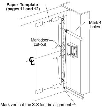
Note: Line X-X is a reference line on the paper template used for trim and exit device alignment. Line X-X shown here should correspond to line X-X in the trim installation instructions
