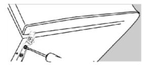
7. Check that the door is aligned horizontally and vertically and that the seals are closed on all sides before finally tightening the bottom hinge.
