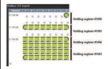
The controller's inputs can also be addressed as coils. The assigned inputs start at coil #1015.
