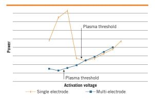
In addition, each electrode has an independent power channel. Current supplied for each electrode is reduced as that electrode forms a plasma layer and resistance increases. This minimizes total current and subsequent power or heat dissipated to collateral tissue.
