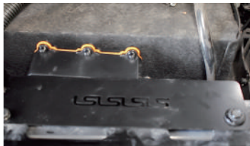
1.3 Mount the bracket(s) with the power distribution.
