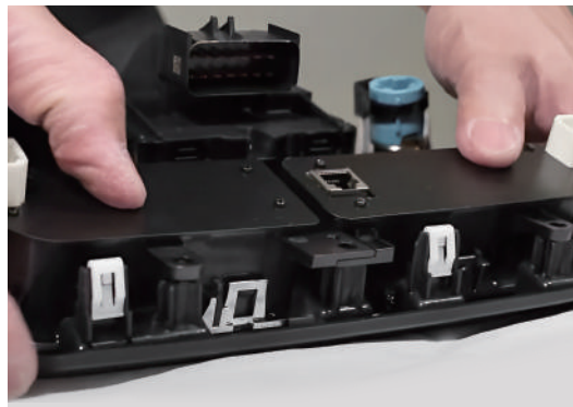
4.2 Install the switches and reinstall those 5.5mm screws.
