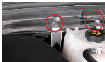
2.2 Disconnect the bolts and run the wires behind the tank.
