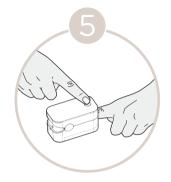
Press button to take measurement. Readings can take up to 1 minute to stabilise.
