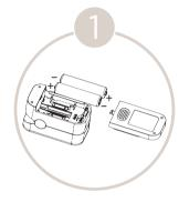
Open battery cover, insert batteries and replace cover.
