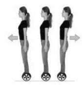
To turn, simply slow down and lean your body left or right. The built-in inertia dynamic stabilization system will maintain the direction frontwards or backwards. However, it cannot guarantee stability while turning left or right. As you drive the Hoverboard, please shift your weight in order to overcome the centrifugal force and improve your safety while turning.
