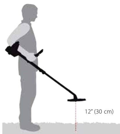
Figure 17 – Correct detector position for Noise Cancel
