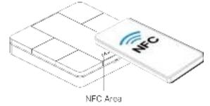
5. Basic information and settings of the device will be shown on ToolBox if it's recognized successfully. You can read and configure the device by tapping the Read/Write button on the App. In order to protect the security of devices, password validation is required when first configuration. The default password is **123456**.
