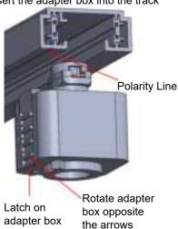
Rotate the adapter box opposite the arrows until the latch snaps in place between the two track rails
