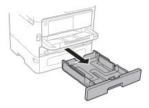
**2** Slide the side edge guides all the way out and set the front edge guide to the paper size you are using.
