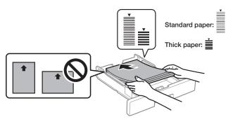
**Note:** Make sure the paper is under the arrow mark for your paper type and loaded against the front edge of the cassette.
