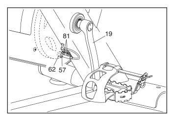
Next, turn the Left Crank Arm (19) until a Magnet (62) is aligned with the Reed Switch (57). Slide the Reed Switch slightly toward or away from the Magnet. Then, retighten the M4 x 16mm Screws (81).
