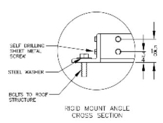
Figure 17 - Seismic Rigid Mount Curb
