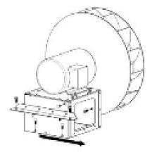
Figure 39 - Bolts which Connect Motor Mount to Blower Fan
