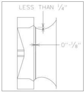
Figure 28 - Plenum Fan Gap Tolerances
