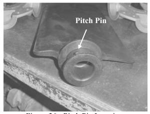
Figure 36 - Pitch Pin Location
