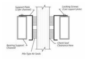
Cross Section of Air Seal Structure
