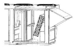
Figure 42 - Evaporator Coil Access
