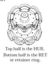
Figure 32 - Fan HUB and RET Castings
