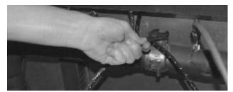
4. Remove the bolts from the suction filter end plate
