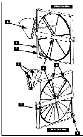
Figure 47 - Polymer Energy Recovery Wheel
