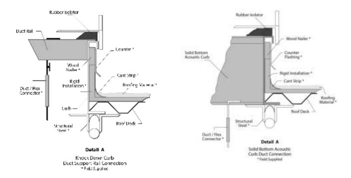
Figure 12 - Duct Connection
