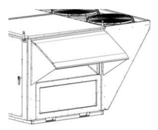
Figure 19 - 11, 13 and 16-30 ton Open Rain Hood
