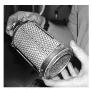
Figure 44 - RPE-48-BD filter element
