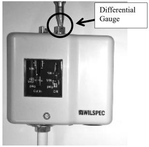
To lower the pressure set point for the **DIFFERENTIAL** Gauge, turn the adjustable screw counter clockwise.
