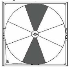
Figure 48 - Wheel Segment Removal Pattern
