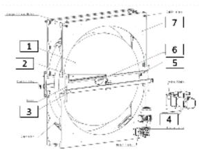
Figure 45 - Aluminum Energy Recovery Wheel
