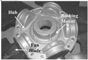
Figure 33 - Assembled Fan
