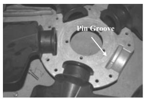
Figure 35 - Pin Groove Location
