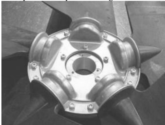
Figure 34 - Back of the Fan
