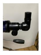
Loosen the thumbscrew.Insert the eyepiece into the diagonal lens.
