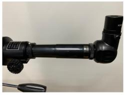
10. If there is a balow len,insert it between eyepiece(diagonal lens)and the focusing tube. Maybe it's better effect between eyepiece and focusing tube without diagonal lens. Depending on your need
