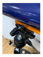
4. Put the astronomical body into the tripod head and turn the screw knob to fix it.
