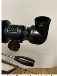
8. Insert the diagonal lens into the focusing tube. Hold it in place by tightening down the mounting bolts
