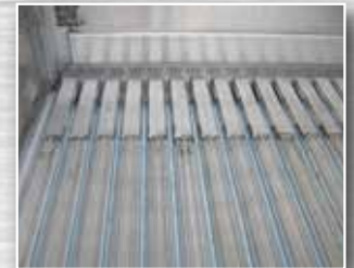
Triple Ridge 18, Slat Floor with 2' Wear Strips at Rear
