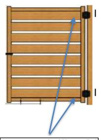
Hinges position should be installed as shown in drawing [3.5 inches from the top and bottom]
