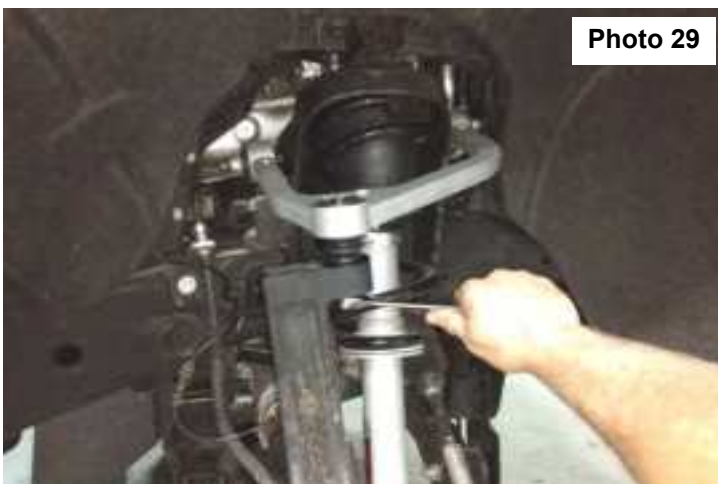
Tighten upper ball joint.
