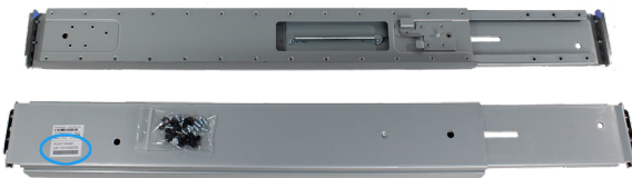
Rail kit and hardware. The rail front ends are labeled. You must install the front ends of the rails facing the front of the rack.
