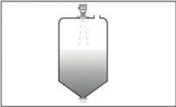
Figure 3: Conical vessel installation
