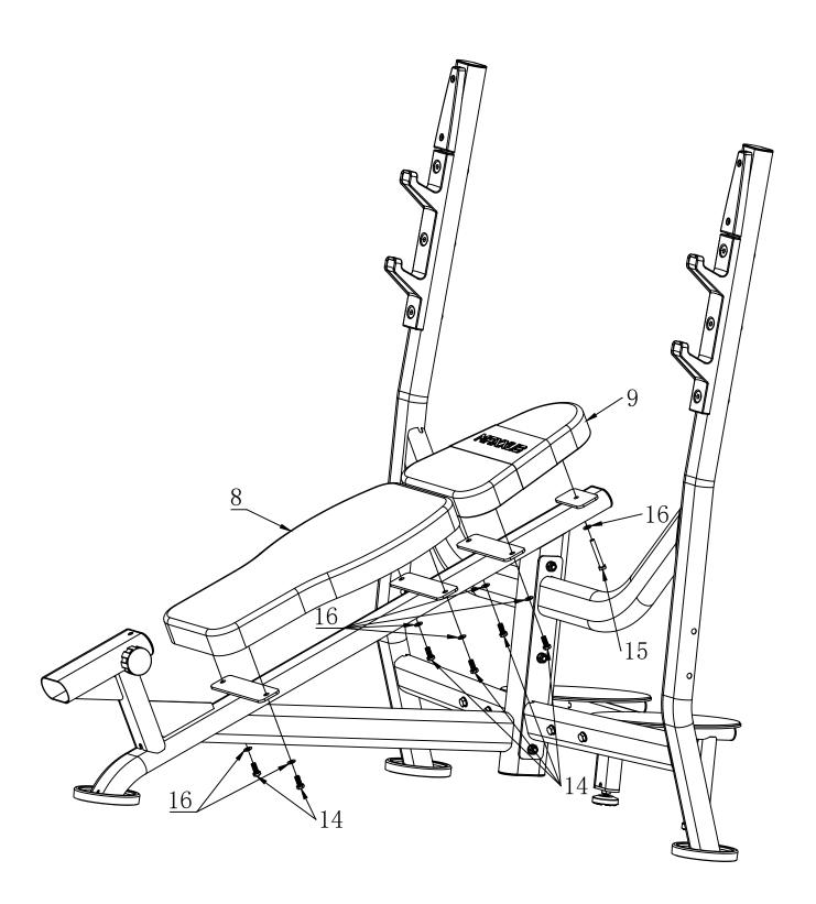
Lock Seat cushion (No.7) into Pre-assembled part assembly (E) with 3pcs External hexagon screw M8\*20 (No.14) and 3pcs Flat washer  $\varphi$ 8 (No.16). Then, insert Pre-assembled part assembly (E) into the hole of Pre-assembled part assembly (C) and lock well with M16 Elastic bolt (No.36) that pre-assembled as shown in the picture.
