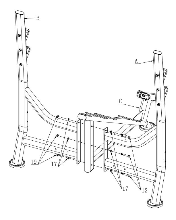
Lock Pre-assembled part assembly (D) into Pre-assembled part assembly (A) and Pre-assembled part assembly (B) respectively with 2pcs Adjustable foot pad (No.32) 4pcs External hexagon screw M10\*60 (No.11) 8pcs Flat washer  $\phi$ 10 (No.17) and 4pcs Locking nut M10 (No.19) as shown in the picture.
