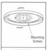
Secure fixture by tightening mounting screws.
