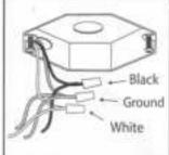
Using wire nuts to connect ground wire (green) from fixture and LED board to ground wire from electrical box.
