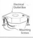
Place mounting screws (included) in electrical box screwing in halfway.
