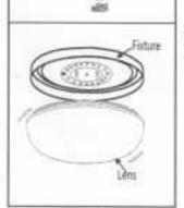
To install acrylic plastic lens, hold lens up to fixture, and rotate until notches in lens line up with tabs in fixture.
