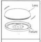
Remove plastic lens by gently rotating and lifting.
