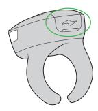
Open the mudflap to expose the charging port.
