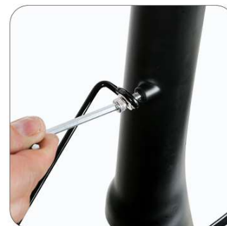
Tighten the screws on right sides of the front fork
