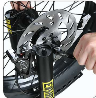
After screwing to a certain strength, fasten the quick release handle in the direction of the arrow
