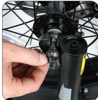
Tighten the spring and nut to the screw
