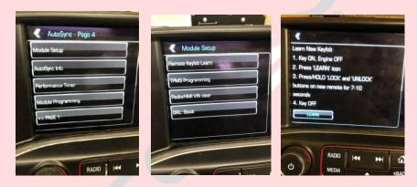
Module Programming – This menu option is to enter module reprogramming mode, to flash custom third-party tuning into the BCM, HMI module, and radio. Custom BCM tuning can unlock additional features such as speed limiter disable, remote-start timer extend, disable LED turn signal hyperflash, and MUCH more!
