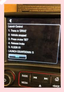
NOTE: It is strongly advisable to NOT use launch control repeatedly, and you should allow several minutes' cool-down time for the ABS pump motor and ABS solenoids between launch control events. Repeatedly/continuously using launch control MAY cause premature wear on the ABS pump motor and solenoid valves.
