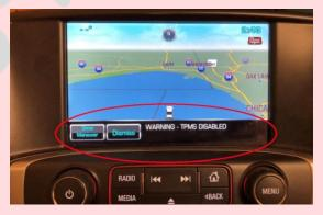
NOTE: when the AutoSync is set to disable TPMS, the truck will still chime and display a temporary "TPMS DISABLED" message on the radio/navigation screen after startup. This is simply to warn the driver that TPMS has been disabled by AutoSync. **Do NOT press "Show Maneuver" or "Dismiss", this on-screen TPMS warning message will automatically self-clear within 5 seconds.**
