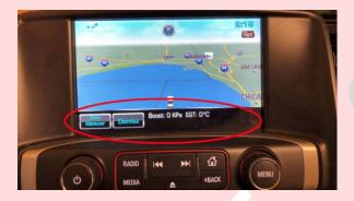
Due to the smaller size of the "minimized" view, only two PIDs are able to be displayed at once in this mode. To cycle through the pages of minimized data display, press the drivers door lock button. To switch back to the engine data full page, press the "Show Maneuver" icon.
