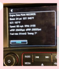
**NOTE:** the "EGT" reading is derived from the factory "EGT-1" sensor, located in the factory downpipe at the outlet of the turbocharger (LML) or "EGR-1" in the manifold (L5P). **If this sensor is unplugged or removed due to an aftermarket downpipe, EGT will not display correctly and will default to "1832\*F".** If your truck is 'deleted', you can extend the factory sensor wiring and re-locate the factory EGT-1 sensor to the exhaust manifold for a more accurate "pre-turbo" reading.
