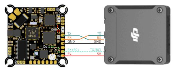
The supply voltage is fixed 5 V. Make sure your VTX and additional Peripherals do now draw more than the <u>built-in BEC (on page 28)</u> can provide.
