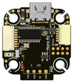
RX4 - SBUS IN GND RX3 - OSD TX3 - OSD GND VBAT/ 9V
