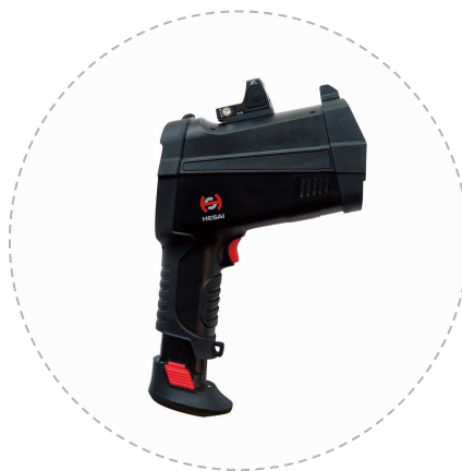
Step2 Pull the battery out gently Figure 4.4 Remove Battery Steps
