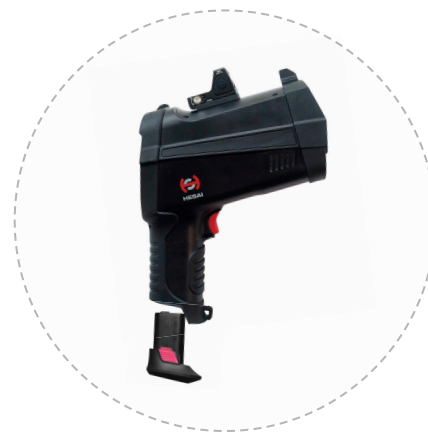
Step3 Till the battery is fully unplugged
