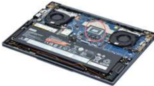
Figure 4. Areas on the system board where thermal interface materials are applied
