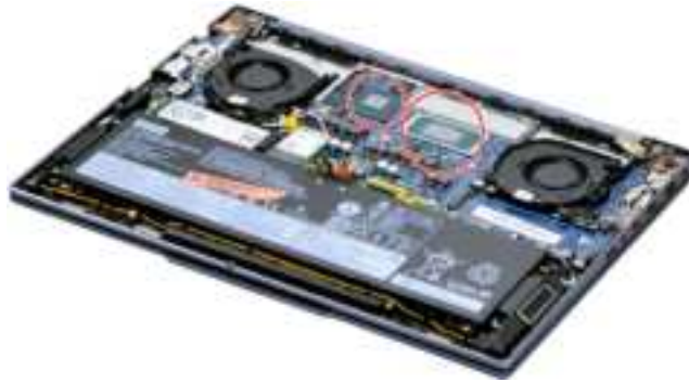
Figure 8. Areas on the system board where thermal interface materials are applied
