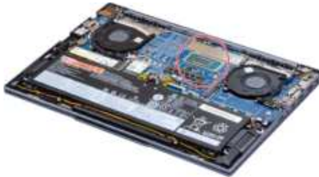
Figure 6. Areas on the system board where thermal interface materials are applied
