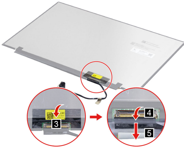
Figure 49. Remove the EDP cable
