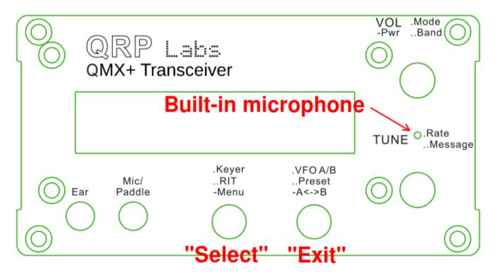
The front panel of the QMX+ has the same controls but they are arranged differently in a Desktop transceiver format, as opposed to QMX where the controls are on the top face of the unit which is more suitable for portable operations.
