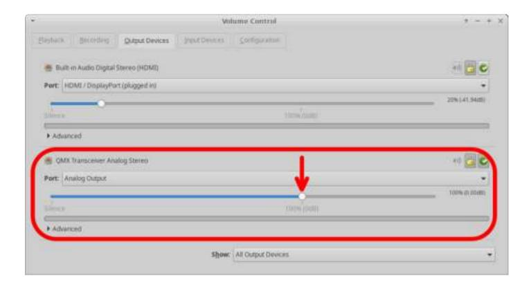
3. The "Master Volume" control of the PC should also be set to 100%. There is such a setting in both Windows and Linux (and most likely Mac too). In Linux, clicking the loudspeaker icon at the bottom right of the screen shows which audio device is being used for the default sound output; selecting QMX will show you the master volume level, and it needs to be set to 100% (not more, not less). There's a similar thing on Windows OS.
