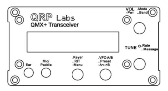
This is the front panel of the QMX+. The Earphone and Mic/Paddle 3.5mm connectors are on the FRONT panel of the QMX+. The pinouts are the same as for the QMX (described above).
