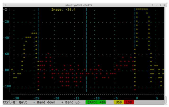
You may get better or worse image rejection than this (depending on your particular combination of component tolerances) and toroid winding style. This is not normally something to worry about.
