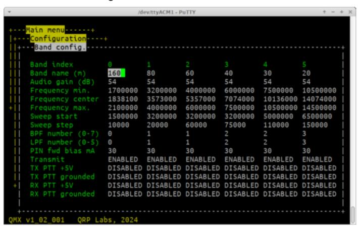
The Band Configuration screen allows specification of all parameters that are handled per-band. This screen is populated by default with the correct information to set QMX up for 5-band operation on 80, 60, 40, 30 and 20m (See above). However, if you wish to experiment with other bands (which will require hardware modifications to Receiver Band Pass Filter and Transmitter Low Pass Filter component values – for which you are on your own), then you may specify the other band parameters here.
