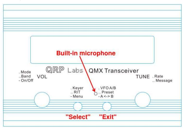
This diagram shows the operating controls of the QMX. There are two rotary encoders at left and right, and two push-buttons in the center. The main function of the left rotary encoder is Volume adjustment, and that of the right rotary encoder is Tuning. However, all of the controls have multiple functions, depending on the operating mode, menu editing, etc. The rotary encoders both
