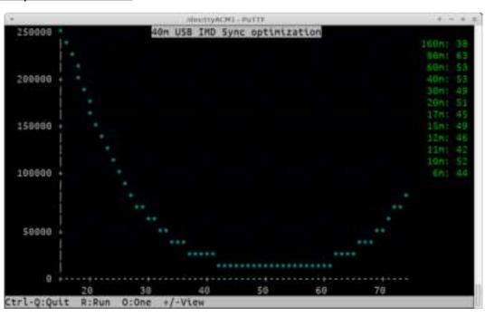
synchronization setting, and is entered into the table of synchronizations on the right hand side.
