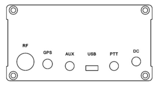
This is the rear panel of QMX+. The RF, USB, PTT and DC connectors are exactly the same as described in the section above. The Paddle/Mic and Earphones connectors are on the QMX+ front panel (see below).
