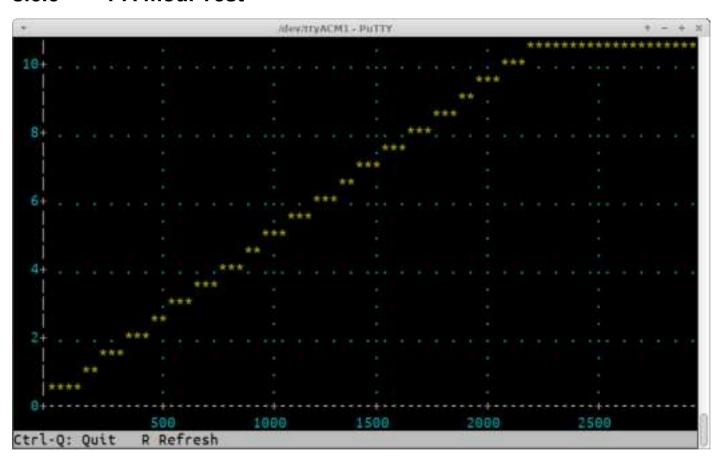
The PA amplitude modulator test screen increases the DAC voltage applied to the amplitude modulator (X-axis) while measuring the resulting voltage supplied to the PA (Y-axis). It should be a very straight line going from near the bottom corner, to near the positive supply voltage.
