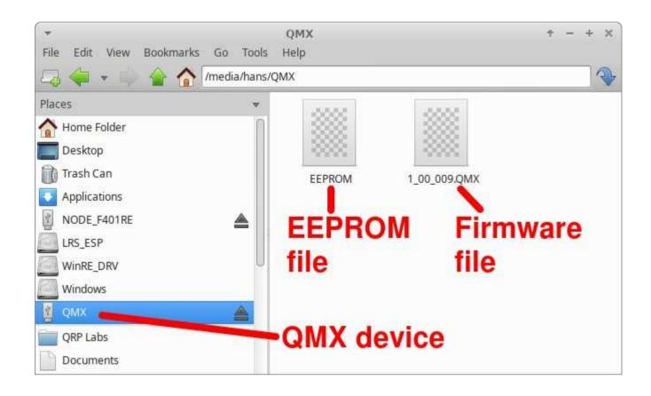
QMX appears as a removable USB Flash device named "QMX", and the folder two files. The firmware file in this example is named shows a single file which is the firmware version file, 1\_00\_009.QMX in this example. The EEPROM file is always named EEPROM. You can read and write EEPROM files in order to make and restore backup copies of your configuration etc.
