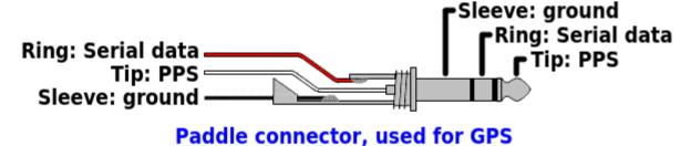
Here the 1pps signal from the GPS must be connected to the 3.5mm jack "tip" connection, and the serial data (9600 baud) to the "ring" connection. In QMX these signals are 3.3V logic level; however they are connected to 5V-tolerant I/O pins on the microcontroller so 5V logic level will also work fine. If you are using a GPS module directly, and it has the common 2.8V output logic, this will also work fine.
