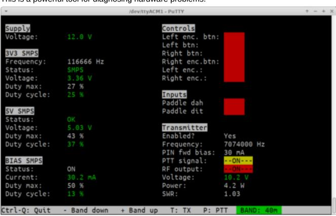
Several areas of the screen show a colour coding. Green means the operation is correctly within allowable parameters, and it's a "PASS". Red means the operation is outside allowable limits, or that the function has not been tested yet.
