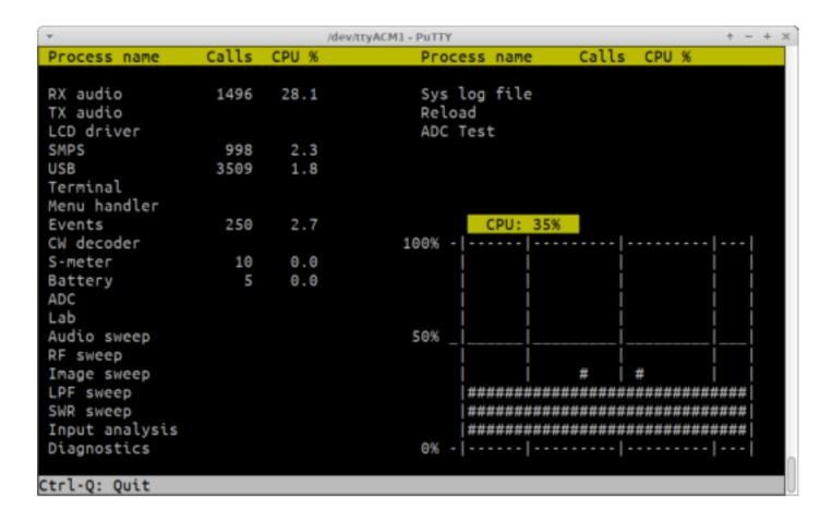
The primary use of the CPU Monitor tool is for firmware development purposes, to make sure that processes are not being called unnecessarily, are not taking up more CPU time than they should, and to investigate improvements to the efficiency of various processes in the system.
