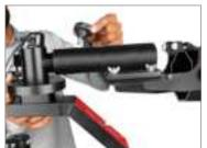
• The Spin-3 Pan-Tilt Head is securely attached to the mounting plate.
