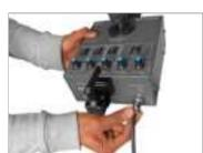
• Connect the AC Adapter's female end to the Joystick controller.
