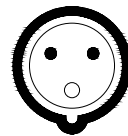
IEC 60309, 2P+E 6H 3W IP44 (SPLASHPROOF) 32A, 200-250V MAX RATED INPUT
