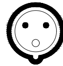
IEC 60309, 2P+E 6H 3W IP67 (WATERTIGHT) 32A, 200-250V MAX RATED INPUT
