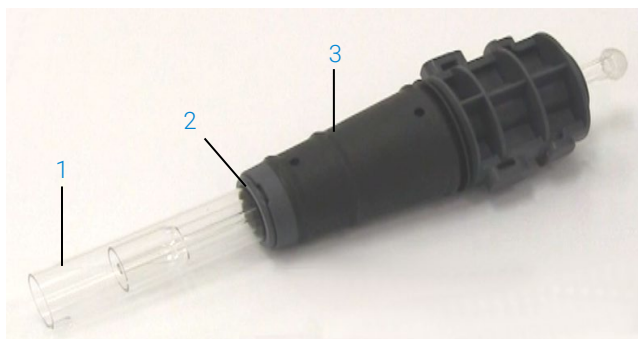
Figure 3. Demountable torch where: 1. Torch, 2. Top seal and 3. Torch body
