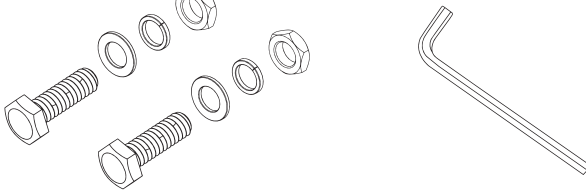
2 x M8 Hex Head Screws (L25) 2 x M8 Washers 2 x M8 Spring Washers 2 x M8 Nuts
