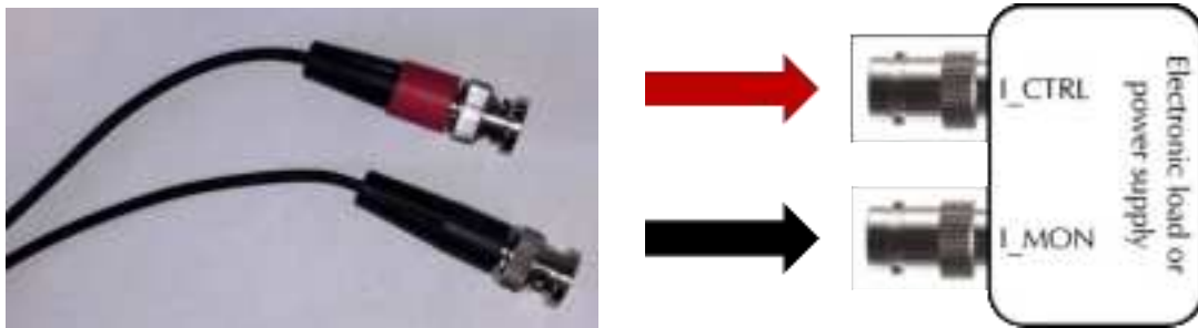
Figure 4-5 Schematic overview of current control (I_CTRL) and current monitor (I_MON) cable installation
