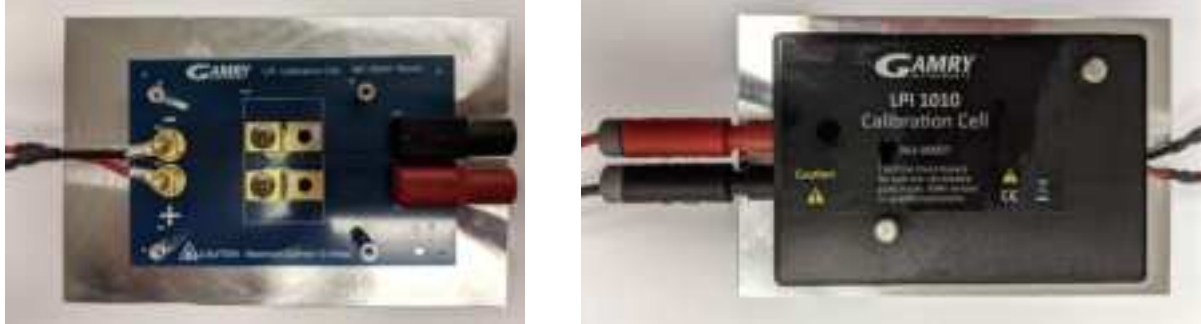
Figure 5-7 LPI1010 200 mΩ Calibration Cell with connected cell leads
