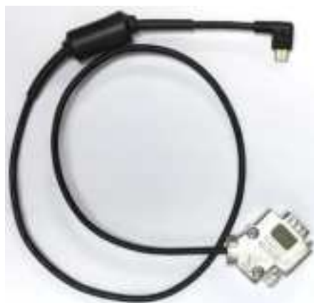
Figure 4-3 LPI Power Cable
