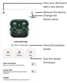
» Device name: To edit your earbud name, tap \( \int \) Edit icon in the top right of the screen. » Battery levels: To view the battery levels of both the charging case and earbuds, put both earbuds into the case.
