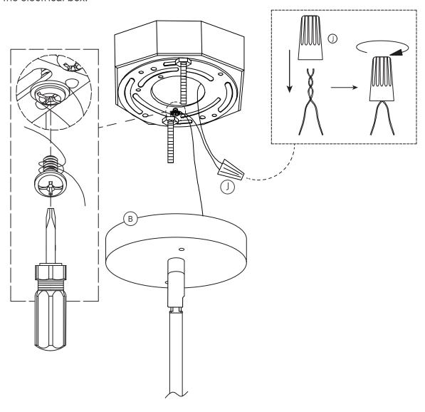
Use the Wire Connectors (J) to join the remaining matching colored wires (White to White, Black to Black). Once complete, tuck the excess wire into the electrical box.
