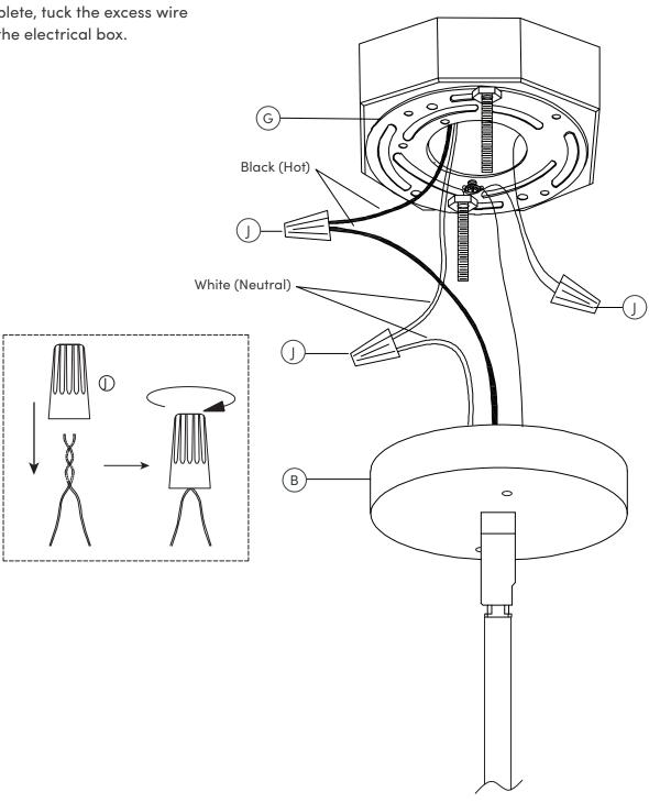
Secure the Ceiling Plate (B) to the Mounting Plate (G) on your pre-installed electrical box using the Finial Nuts (H) that you originally removed in Step 1.
