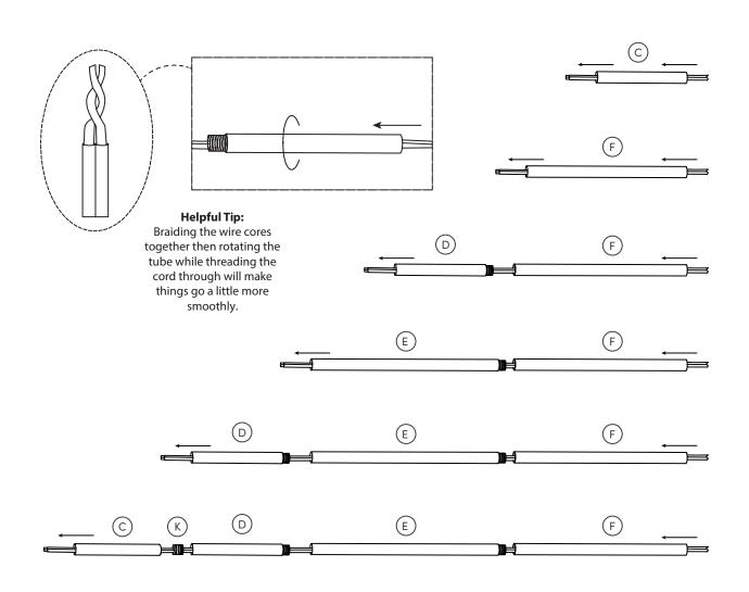
Thread the necessary stem components together to complete the connection between the Canopy (B) and the Shade assembly (A).
