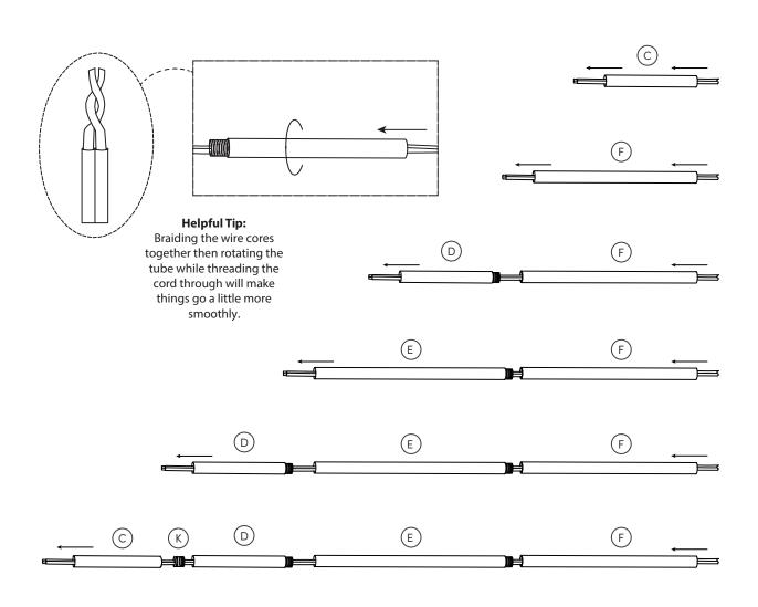
Thread the necessary stem components together to complete the connection between the Canopy (B) and the Shade assembly (A).
