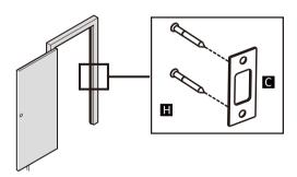
IMPORTANT: Make sure hole in door frame is drilled a minimum of 1" (25 mm) deep.
