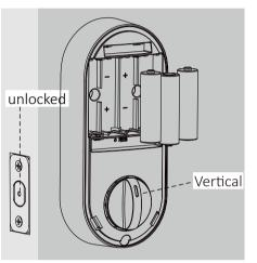
While the door is **OPENED** and **UNLOCKED** (latch retracted), load 3 AA batteries into the battery compartment.
