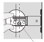
Slotted hole is NOT centered. Rotate and pull the latch as shown to extend latch.
