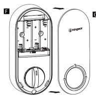
Locate the slot at the bottom and use your fingernail or a flat head screwdriver to pry the cover up and pull it off.
