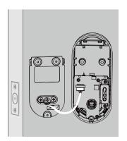
Insert the cable connector to the socket. Push the connector in firmly until it is completed seated.
