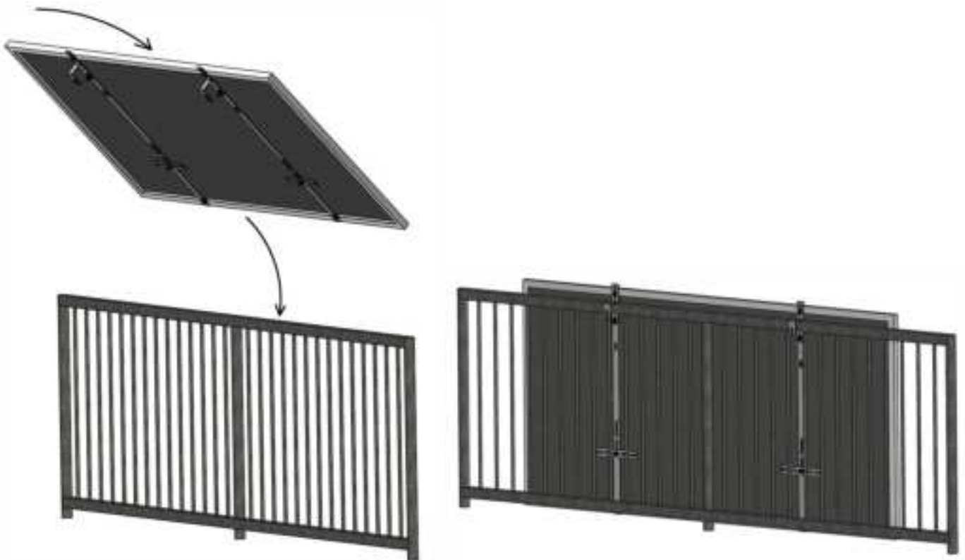
FIG.7 Installation of the structure on the railing
