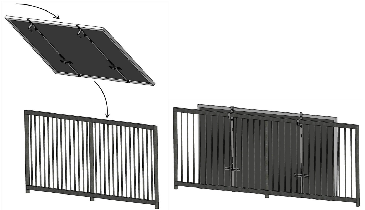
FIG.7 Installation of the structure on the railing
